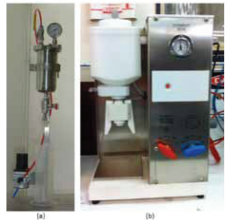
Figure 1. Different types of apparatus for measuring FI: (a) manual equipment; (b) semi-automated equipment.
