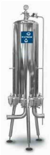
The DISCSTAR™ P is an economical stainless steel filter housing for lenticular depth filter modules. The enclosed system allows high capacity depth filtration with no drip loss (no edge leaking). Designed and manufactured for heavy duty use – 24/7. System of choice for frequently changing filtration applications in the pharmaceutical industry. This system provides pressure stability up to 10 bars.
