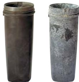
No corrosion with Alocrom treatment.
