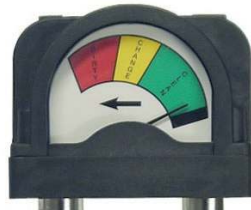
Differential Pressure Gauge
