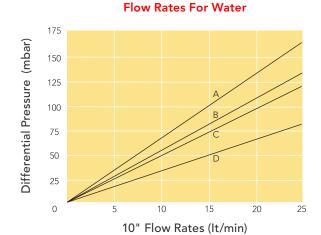
A=0.05μm B=0.1μm C=0.2μm D=0.45μm/1μm
