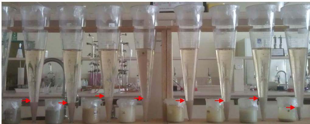
Settling kinetics: SIHA Active Bentonite G settles rapidly
