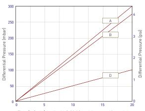
Flow (L / min) for liquid @ 20 °C and 1 cp per 10"module Recommended wine flow rate 10L/min/10" module
