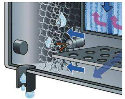
The **SmartDrainer** is fitted in models PST120 and upwards. The draining chamber is integrated into the heat exchanger, while the valve mechanism is located in an easily accessible drain niche.
