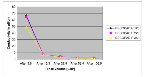
The conductivity of the extract was < 20  $\mu$ S/cm after a rinsing volume of 22.9 l/m<sup>2</sup> and can be lowered further by additional flushing.
