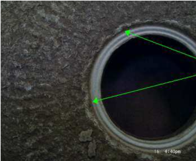
Image taken of market leading competitors module that is pressed too hard and therefore caused damage to the media.
