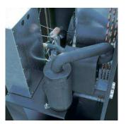
The pneumatic circuit, including a heat exchanger with copper brazed plates and condensate separator, is made of stainless steel to increase resistance to corrosion, which is common in certain environments and processes.
