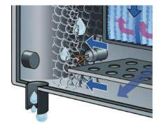
The **SmartDrainer** is fitted in models PST120 and upwards. The draining chamber is integrated into the heat exchanger, while the valve mechanism is located in an easily accessible drain niche.
