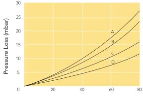
Air Flow Rates (m<sup>3</sup>/hr @ 0 barg) A=0.3μm B=0.5μm C=1.0μm D=5.0/10μm
