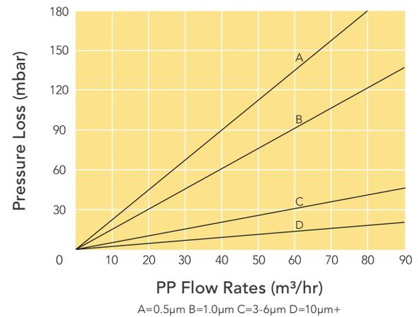
\*1 Amazon Filters recommend that SupaPleat HFC SRP cartridges are changed at a differential pressure of 1.5 bar in normal service - the operating conditions above should be treated as maximum differential pressures for short term use without causing cartridge collapse problems.
