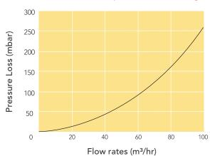
For total pressure drop values for final assembly add media pressure drop to fixed pressure drop
