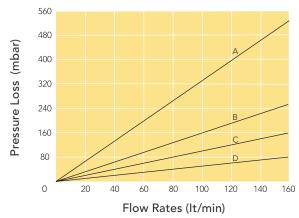
A=0.5μm B=CRY/1.0μm C=2.5/5μm D=XP/10μm+
