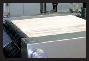
At the end of the filtration **BECOPAD** shows no more than slight discolouration: no drip losses.\*
