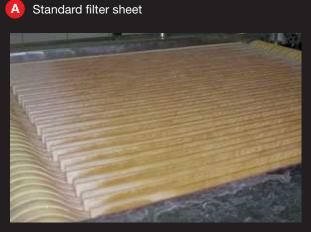
Conventional depth filter sheets tend to become stained quite quickly – a possible indication of drip losses.
